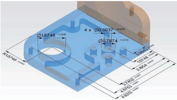
This includes a new right-click configuration tool used for diameter, radius, slot dimensions and distance between annotations allowing precise position of GD&T dimensions.
