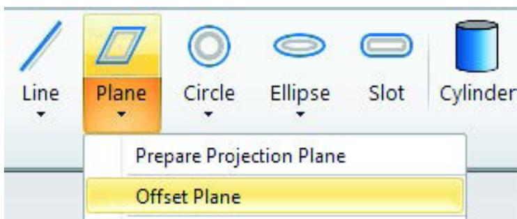
Allows a user to select an existing plane and the relationship maintains the specified distance from that reference plane.
